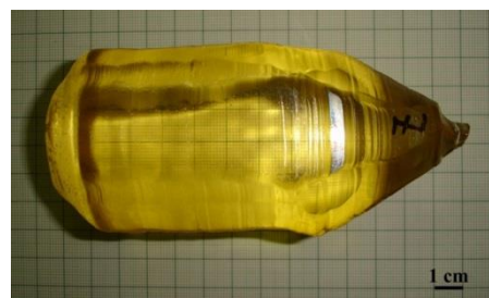
3" ordered \text{Ca}_3\text{TaGa}_3\text{Si}_2\text{O}_{14} crystal.
