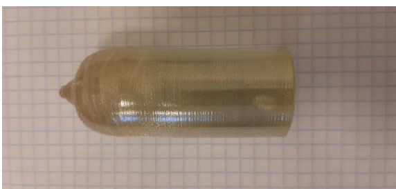
\text{LiNb}_{0.88}\text{Ta}_{0.12}\text{O}_3 crystal grown by the Czochralski method along axis c .
