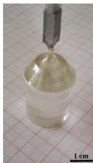
\text{LiNb}_{0.93}\text{Ta}_{0.07}\text{O}_3 crystal grown by the Czochralski method along polar axis c .
