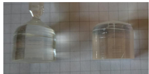
Fig. 3. LiNb_{0.88}Ta_{0.12}O_3 crystal grown by Czochralski method with a very low pulling rate.
