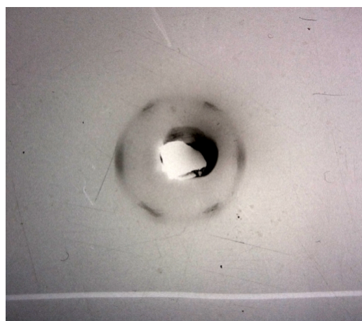
Fig. 5. The X-raygram of the concentrated sample of AOT-water.
