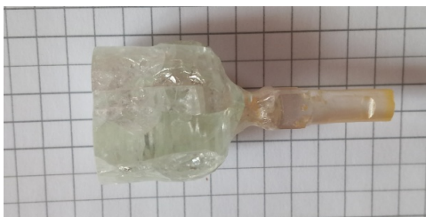
Fig. 2. LiNb_{0.88}Ta_{0.12}O_3 crystal grown by conventional Czochralski method.
