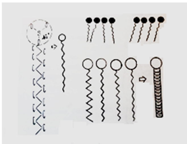
Fig. 2. Schematic structure of the PDSN molecule and its arrangement in the lamella
