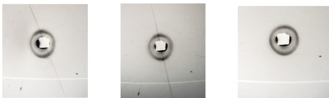
Fig. 3. The radiogram of 86% samples of the PDSN–PEG–water system with the content 9% PEG at temperatures of 308, 313, 353K.
