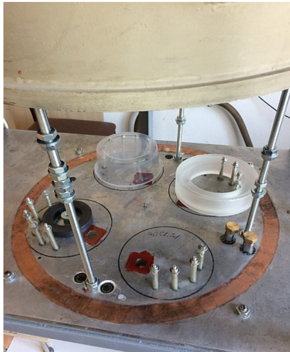
Fig. 3. The working surface of the lower part of the vacuum chamber
